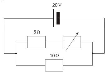
The resistance of the variable resistor is gradually increased from zero to  $5\Omega$ .
