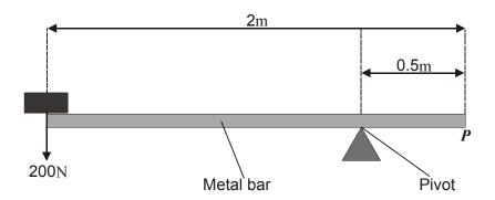
What weight is needed at position *P* to balance the bar?
